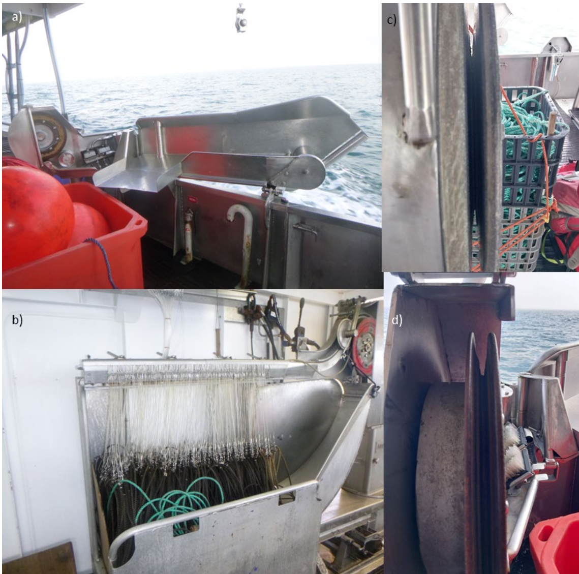
Figure 2. Images of gear and hauler: a) roller with main fishing line hauler on left, b) secondary hauler and hook storage, c) main hauler showing gap between sheaves, apparently worn, d) float line hauler showing smaller gap between sheaves for comparison.
