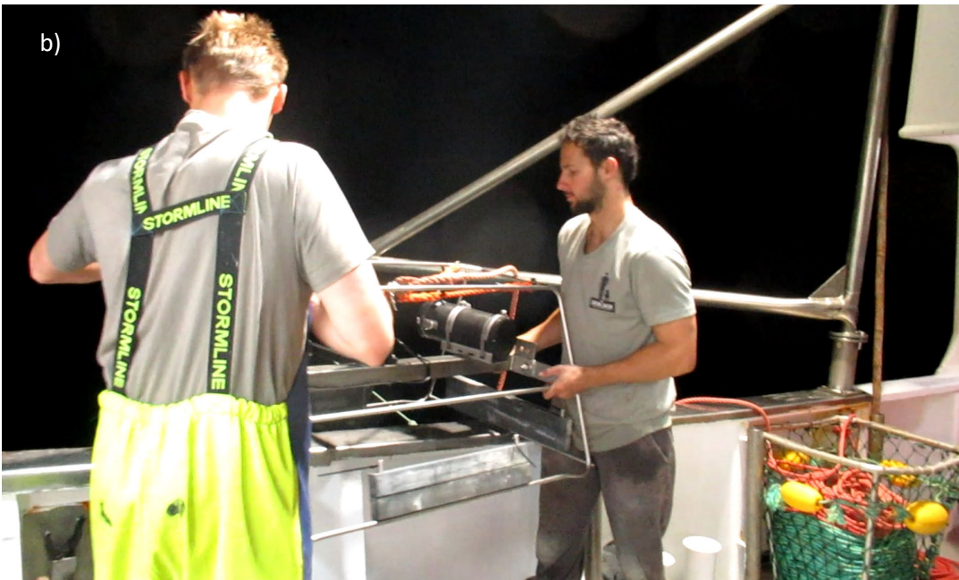
Figure 2 Conventional BRUVS unit deployed during the longline surveys. A). BRUVS unit showing two cameras and a light on a steel frame, with weights and a bait arm; b). Deployment of the BRUVS unit by fishing crew showing the surface rope basket.
