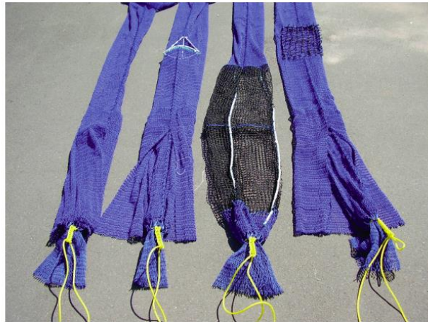
Figure 23: Four BRD ‘treatments’ compared during the trial. From left to right BRD’s were the standard codend with no BRD (control), fisheye BRD, square mesh codend BRD and square mesh panel BRD. The most forward edge of each device was 50 meshes from the drawstring (Source: Courtney et al, 2010).
