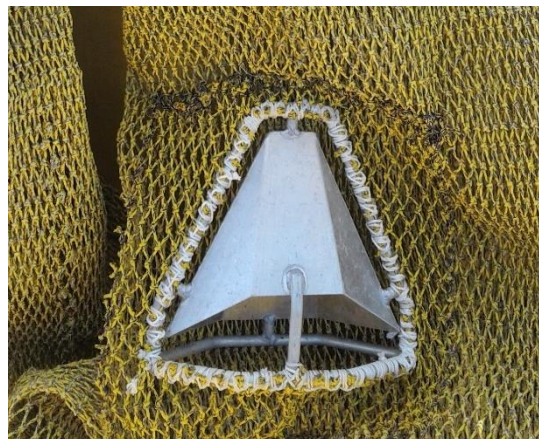
Figure 17: The Tom's Fisheye bycatch reduction device (BRD)
